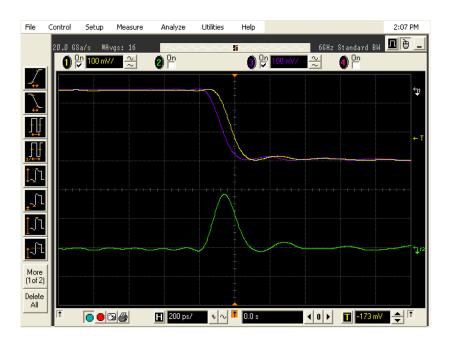
The following picture shows the desired effect of no skew between the cables. Note that the channel 1 (yellow trace), channel 3 (purple trace) traces overlap, and the differential signal (green trace) is flat. If this is not the case, then perform the following steps to reduce the skew between channels 1 and 3.
